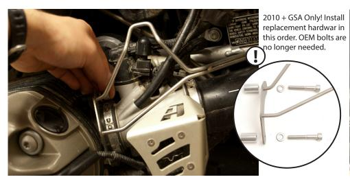
Place the Injector Protector as shown, and start the OEM torx fasteners with your fingers, do not tighten these down just yet. When installed with GSA stand off kit, injector guards may touch potentiometer guard.
