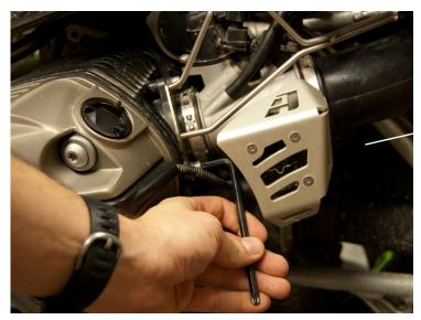
Now you can use your T-30 torx tool to finish tightening the (2) OEM fasteners. For GSA install, consider routing allen key behind the vent line for upper bolt and routing allen key behind the pot guard for lower bolt.
