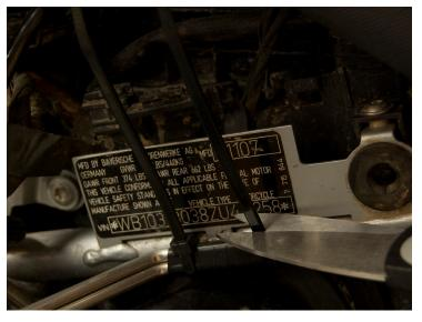
6 After tightening both zip ties, you can snip off the excess.
